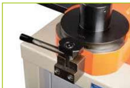
Fast system of die flanges locking
