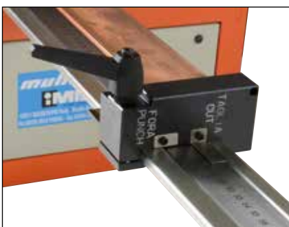
Adjustment distance for punching and cutting.
