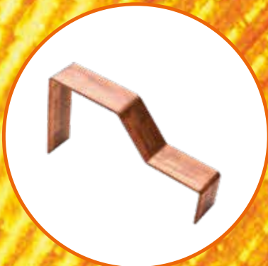
EXAMPLE OF MULTIPLE BENDING
