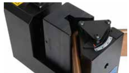
Integrated protractor indicator
