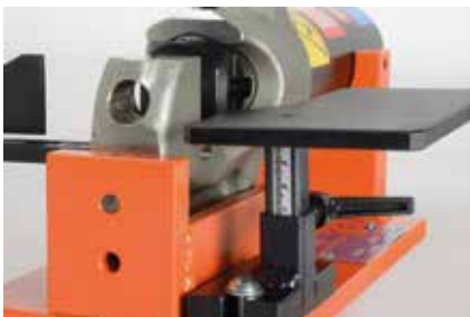
References with millimetric ruler for the right bar positioning.
