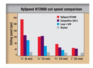
The HySpeed HT2000 and HySpeed HT2000LHF oxygen plasma cutting systems now utilize Hypertherm's patented Coaxial-assist™ jet technology to boost cutting speeds as much as 50% over conventional designs. The Coaxial-assist technology is available at 200 amps using LongLife oxygen processes to cut mild steel from 1/4-inch (6 mm) to 2-inch (50 mm) thick. Dross is minimized and super weldability of the cut edge is delivered.
