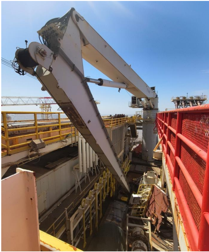
Hydralift Knuckle Boom Combination Crane — Main Boom & Knuckle Jib Detail
