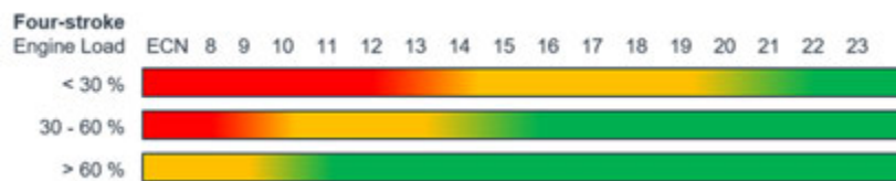
Figure 3: ECN operational reference ranges (CIMAC Fuel quality guide 2011)
