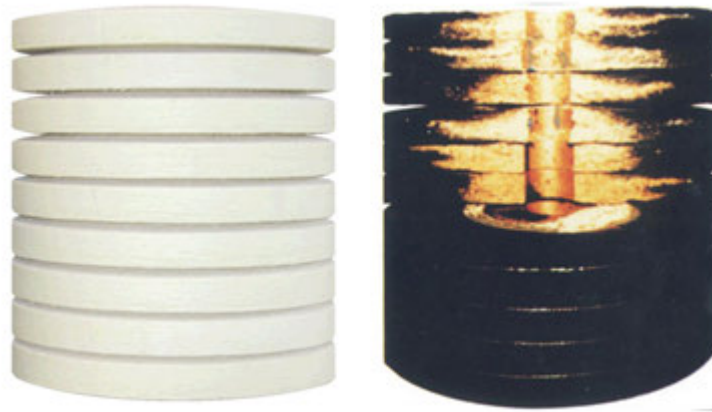
Figure 1: Clean and dirty filter insert
