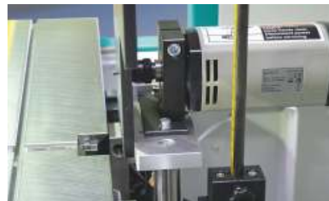
Solid steel guide rods, motor carriage and 1000 watt router motor.
