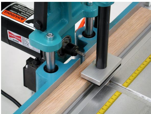
Scrap wood for initial cut through new chip breaker
