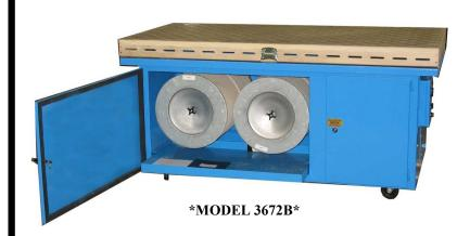
Denray Machines Cartridge Filter System is the best on the market. Denray's "Jet Pulse" pushbutton cleaning line comes in various dimensions to accommodate any job size. These tables all come with 80/20 cartridge filters which clean with a 99.95% capture rate at 0.5 micron.
