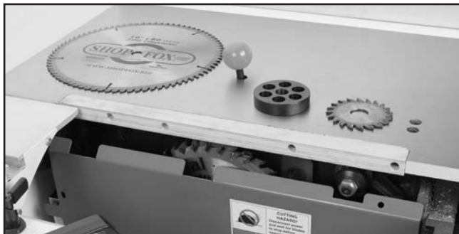
Figure 116. New zero-clearance table insert installed to be cut with a dado blade.
