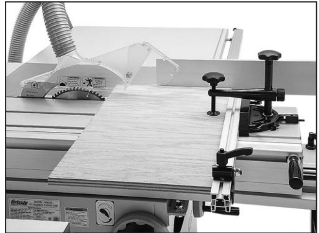
Figure 81. Crosscutting workpieces using the rip fence as a cut-off gauge.
