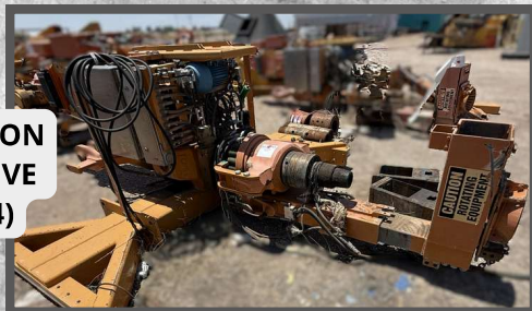
2008 VARCO 500-TON TOP DRIVE SKIDDED
