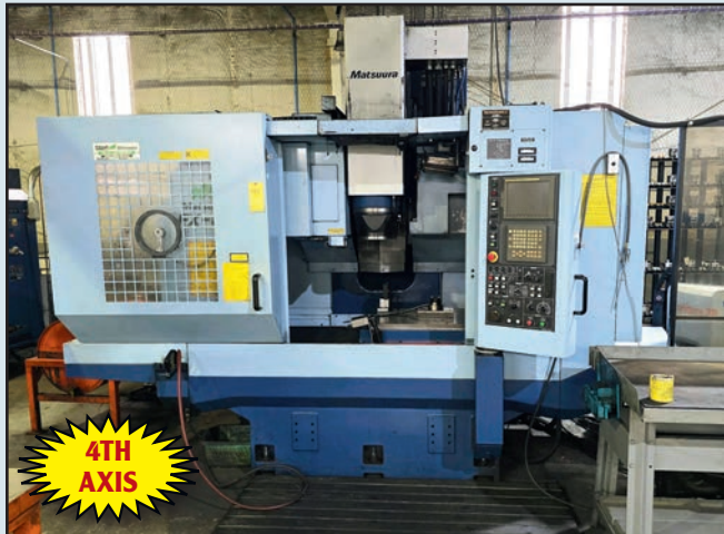
MATSUURA FX-5G VERTICAL MACHINING CENTER WITH AUTOMATION
