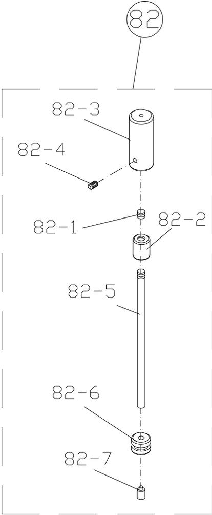
**15.3.2 Spindle Centers Knockout Assembly – Parts List**
