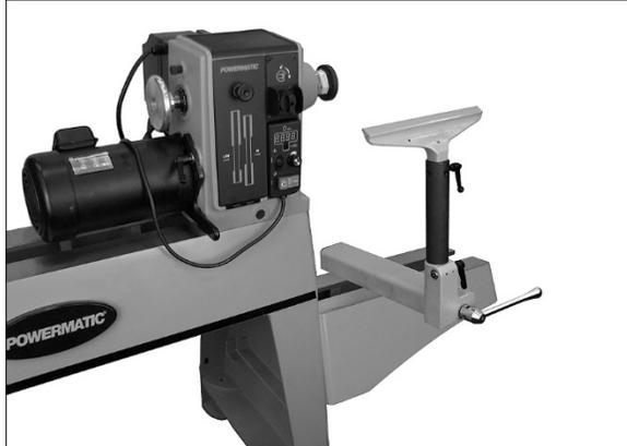
Figure 6-7: outboard turning accessories
