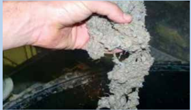
Figure 7: Stringy contaminants can hang up on the rotor foils and form into larger clumps which have the potential to jam between the cylinder and rotor.
