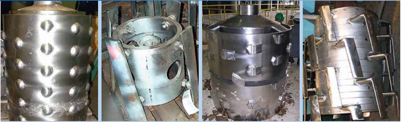
Figure 1: Different rotor designs have come into use since pressure screens were introduced in the 1960s including: a) “bump-type” rotor (1960s), b) “stud-and-nut” foil rotor (1970s), c) “modified bump” rotor (1990s), and d) cantilever foil rotor (2000’s).
