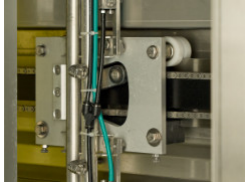
Spray carriage drive unit with sliding clutch
