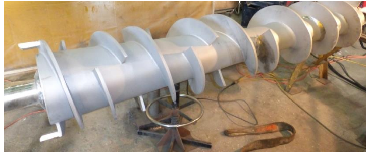
Screw with Tapered (Conical) Shaft
