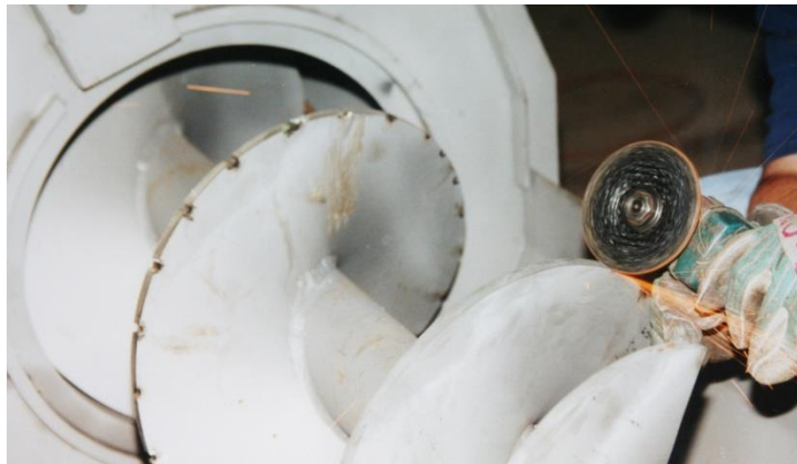
Grinding Notches on Screw Flights
