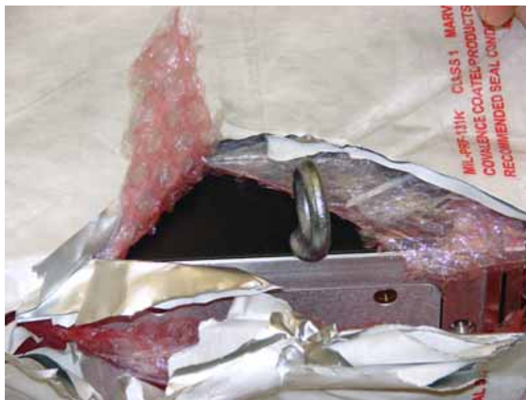
Figure 3-16. Installation of Eyebolts
