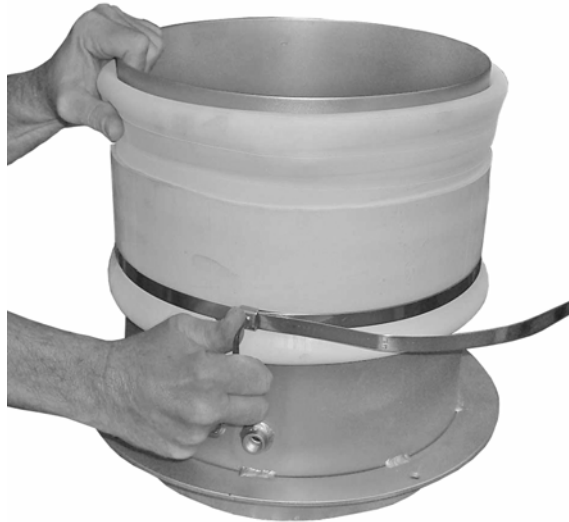
Figure 7-4. Loosening the Setscrew on the Top Compression Ring (Spout Removed From Machine)
