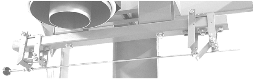
Figure 1-4. Adjustable Locking Bag Strap Hangers (one side shown)
