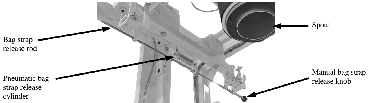
Figure 1-7. Remote Bag Strap and Neck Seal Release
