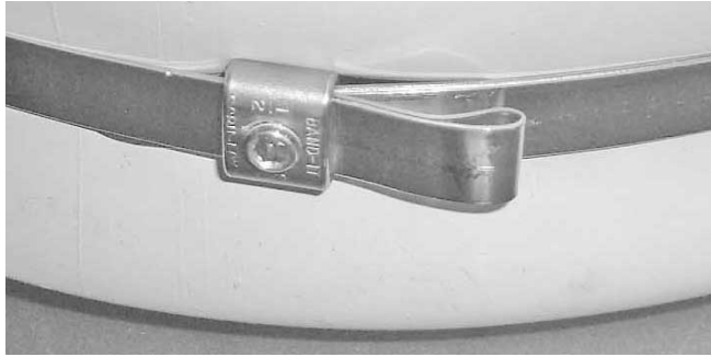
Figure 7-7. Tucking the Excess Compression Ring Under
