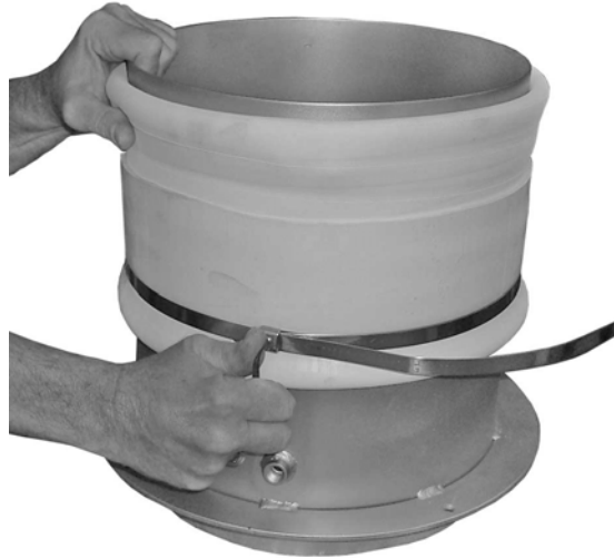
Figure 7-10. Proper Positioning of the Top Compression Ring
