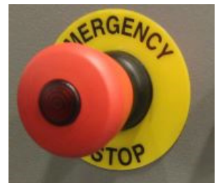
Figure 3-2: Emergency Stop Control
