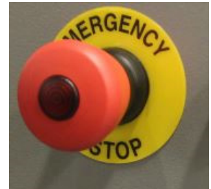
Figure 4-3: Emergency Stop Control
