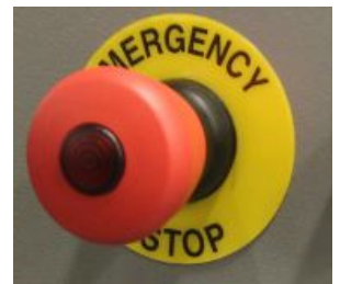
Figure 3-3: Emergency Stop Control
