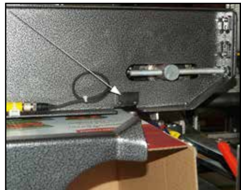
figure 68-3 Case Is Erected Photo Eye
