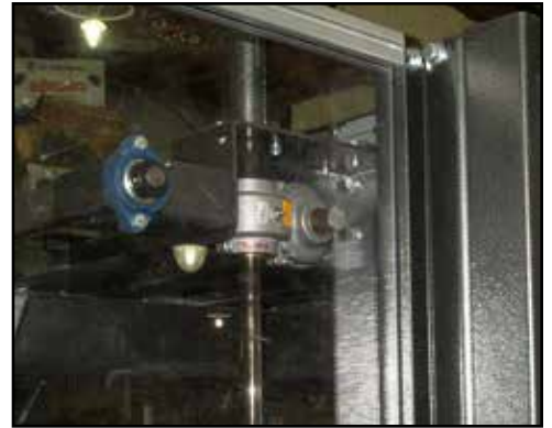
figure 67-1 Grease Zerk on Tolo-Matic Gearcase
