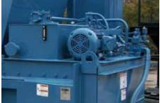
High-efficiency power unit with horsepower limited, pressure compensated piston pump.
