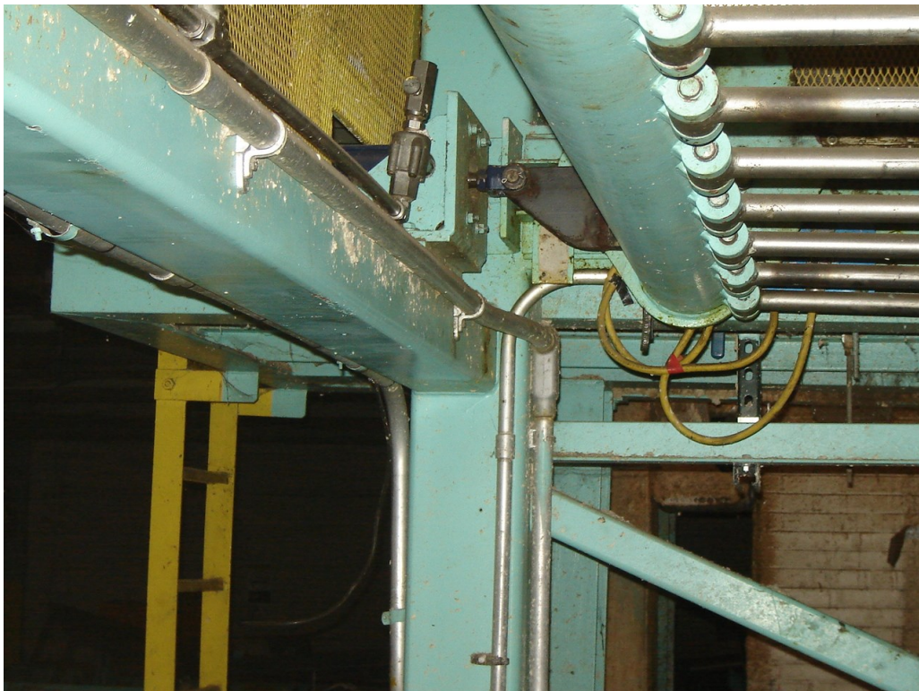
FINGER TABLE - Pneumatically operated, fully automatic. The finger table holds incoming sheets while the stacking table is transferring its load.
