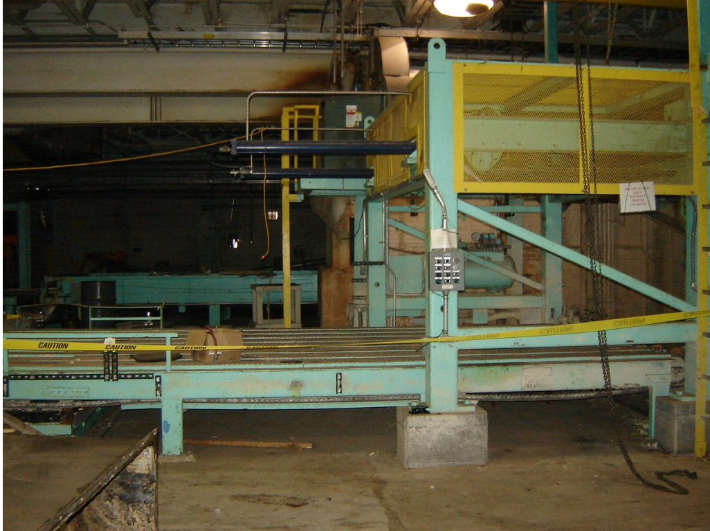
FINGER TABLE - Pneumatically operated, fully automatic. The finger table holds incoming sheets while the stacking table is transferring its load.
