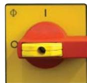
In the event of danger, turn the main switch to "0". You can secure the main switch in this position with a padlock to prevent restarting.
