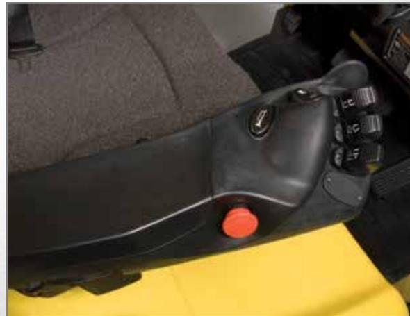
*Electro-hydraulic controls with TouchPoint mini-levers*
