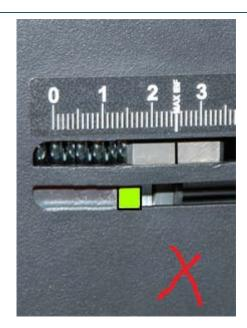
Check belt tension by the indicators on both sides. If the green mark is outside the range of the line, the conveyor should be checked by a trained technician.
