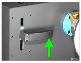
To decrease brake tension, pull the brake handle up.
