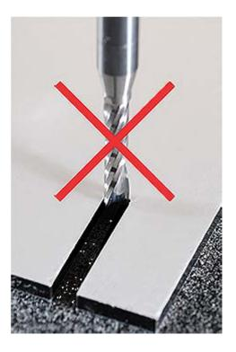
For thin materials, use bits with short **cutting length**.
