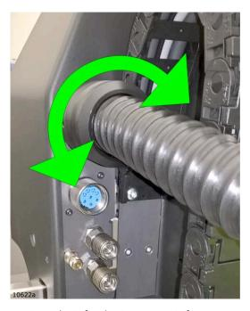
The suction tube is fixed using magnetic force. To release, slightly twist the connector.
