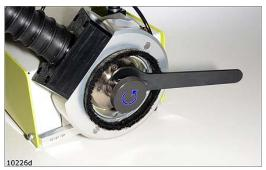
Hold the rotor with the 17 mm key and unscrew the chuck using the **Chuck Tool**.
