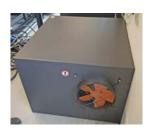
The optional sound insulating box for vacuum pump has a cooling fan with a circuit breaker, which is located in the wall-mounted electrical box.
