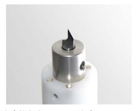
For knife blade change, remove the foot. The locking screw will always point towards the cutting direction.
