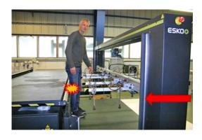
There is a risk of crushing/shearing body parts between moving gantry or pivot arms and support table.
