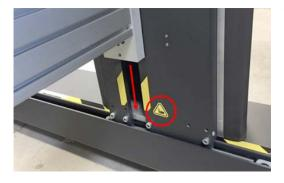
The carriage beam lowers until the plunger sensor detects the top board on the stack.
