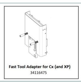
The Fast Tool Adapter makes it possible to attach tools intended for P2 into P1.
