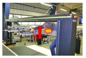
There is a risk of crushing/shearing between moving carriage beam and stack/gantry. Always stop the machine with the dedicated stop control means before accessing the hazardous area.
