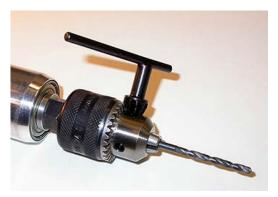
Push the **Drill Bit** towards the bottom of the chuck. Use the wrench to fix the bit in the chuck. No additional adjustments are necessary, as the tool height is measured automatically.
