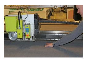
It is possible to reach under the lower DynaGuard light beam into tool hazard areas. Intentionally doing this during machine operation is very dangerous and considered non-intended use.
