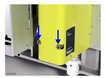
When mounting a tool onto the P1 or P2 **Tool Positions**, ensure that the **Guide Pins** and the electrical connector fits those on the bracket.
