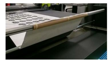
Aligning the media on the Autogrip shaft
