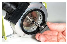
Enter the Chuck Tool with a Dummy Bit into the chuck.
