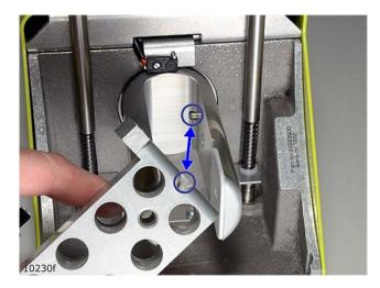
1 Turn the **V-notch Knife Tool** correctly to fit the **Guide Pin**.
