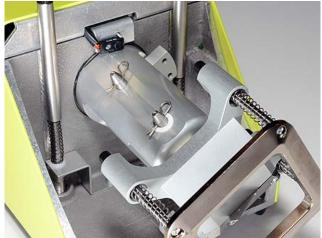
2 Insert the two Latch Pins.3 Insert the Cotter Pins.
