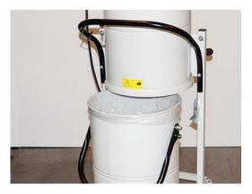
Fold/fix the **Plastic Bag** around the container. Container with **Plastic Bag** ready for operation.
