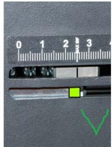
Check the conveyor Y position on the rollers front and rear. The conveyor edge should be close to the middle, short line as shown. If this is not the case, the conveyor should be checked by a trained technician.
