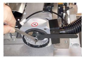
If the bit is stuck, hold the rotor with the 17 mm key and unscrew with a 12 mm key.
