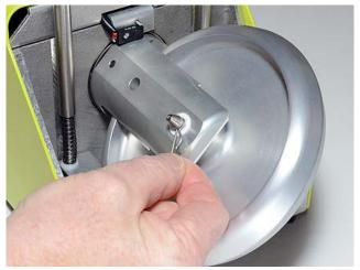
Insert / remove the **Cotter Pin**.
