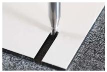
Bits with small **cutting diameter** (3-4 mm; 0.12-0.16 in) are more balanced than bits with larger **cutting diameter**Thus, they can run with higher RPM, normally 60.000.
