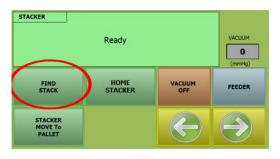
Press the Stacker Find Stack button on the Main Screen.
