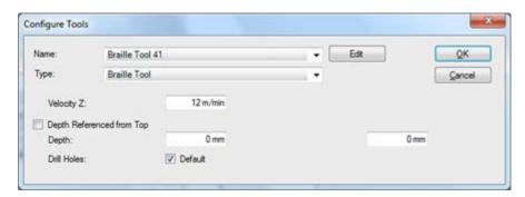
**Braille Tool** should be defined with the following parameters enabled:
