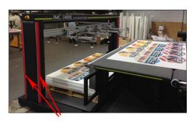
Safety bumpers are located on each side of the moving gantry uprights (arrows) to detect obstacles in the forward or reverse direction of gantry motion.
