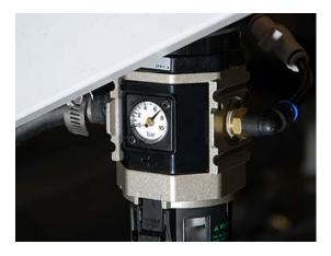
If a **Milling Bit** is stuck in the **chuck**, the probable cause is low **air pressure**.
