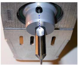
Ensure the knife blade is correctly aligned.
