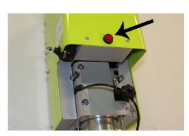
The milling warning lamp indicates that the milling bit is rotating.
