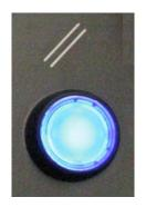
The Fault Reset pushbutton (5) is a blue lighted button.
