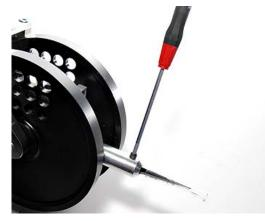
Loosen the fixing screw, replace the knife blade and fix it again.
