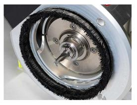
Un-proper **bit clamping** may cause the bit to slip in the **chuck** and damage the **Table Top**.
