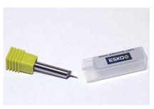
Milling bit edges are brittle. Never let bits touch each other, or other hard surfaces. Always store in proper container.
