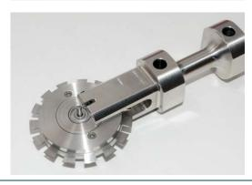
Push/pull the **Perforation Wheel** in/out from the 60 mm crease adapter.
