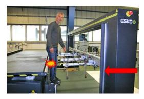
There is a risk of crushing/shearing body parts between moving gantry or pivot arms and support table.
