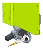
The VariAngle Unit is a tool for position P1 on Ultimate and C/XP platforms. It is specially prepared to cut at different angles (also known as V-notching). The tool can automatically change the angle of the knife between 0 and 60 degrees, in 0.5-degree steps, where 0 degrees is vertical.
