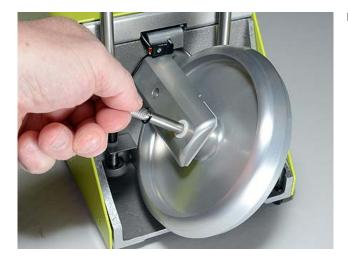
Insert / remove the Latch Pin.
