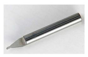
The supplied milling bit is heavily unbalanced and should not be run faster than 20.000 RPM to avoid excessive wear to the milling spindle! This also means that you should not use this bit when warming up the milling spindle as the warm up sequence exceeds 20.000 RPM.
