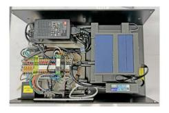
Inside USC Electrical box: PC, Router, encoder, terminal block, power supplies
