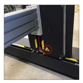
The carriage beam lowers until the plunger sensor detects the top board on the stack.
