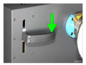
To increase brake tension, push the brake handle down.
