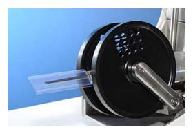
When not in use, protect the knife blade with a knife protector.
