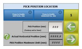
The Pick Position is the location of the gantry where the beam moves down to pick the board from the pallet.
