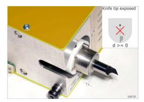
When adjusting the knife tip exposure, do not adjust the knife tip too far into the foot.
