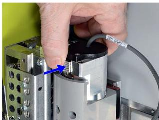
To remove a **Tool** - press the **Release Button**.
