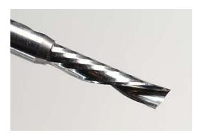
One-flute bits are by nature Non-Balanced, and may destroy the Spindle if used wrong. Therefore, one-flute bits with cutting diameters above 4 mm, 5/32 inch, must be run with a maximum RPM of 40.000 (HPMU)
