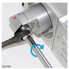
Use the spanner and the hexagonal screw driver to remove the knife blade fixing nut.
