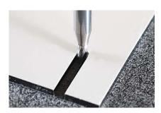
One-flute Bits do have a good chip flow, and allow for large feed rates. 0.1-0.2 mm/tooth (0.004-0.008 in/tooth) can be a starting point for optimization in most materials:
