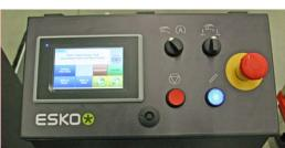
The system has six Emergency Stop push buttons; one located on the pedestal control station, one on each side of the feeder gantry, one on each side of the stacker gantry, and one on the stacker electrical controls enclosure.
