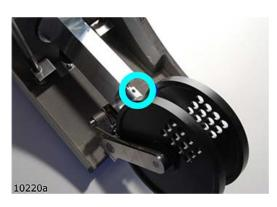
Loosen the fixing screw, replace the adapter and fix it again.
