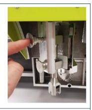
Insert the Locking Pin from one side until it snaps in place. No **Cotter pin** is needed from the other side. For HD inserts other than **HDCrease**, remember to use both pins.
