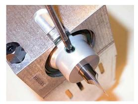
Use a 3 mm allen key to fix/loosen the knife blade.
