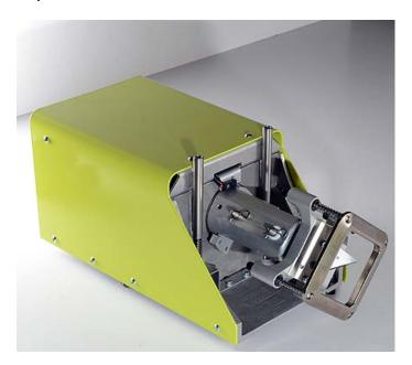
The V-notch Knife Tool mounted on a Heavy Duty Unit.
