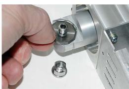
Carefully remove the old knife blade and insert the new one.
