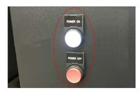
The Power ON / OFF pushbuttons are located on the door of the electrical enclosure.
