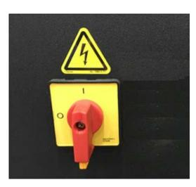
To start up the system; set the Main Disconnect of both the feeder and stacker to the ON position, and then press the lighted Power ON pushbutton located on the door of the feeder electrical enclosure.
