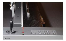
Ensure the traverse safety stop switches are centered.
