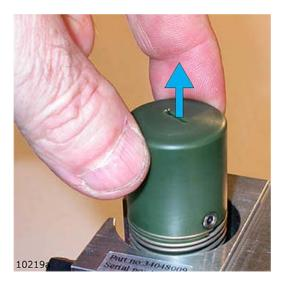
Pull straight out to remove the **Knife Foot**.
