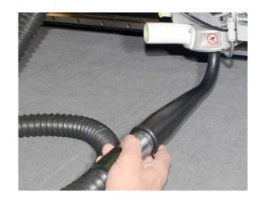
Cleaning the suction house is simple using a **Cleaner Device**, which is available as an option.
