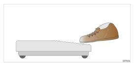
Use the **Foot Pedal** to activate the **Conveyor belt clamp** and **Feeder paws**.
