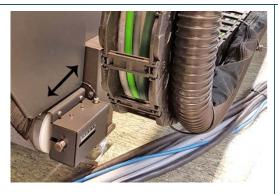
On lower rear roller, there are pneumatic mechanisms for auto-correction of the conveyor position. These will slightly move the roller in and out to corrigate the belt position.
