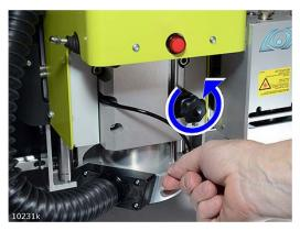
Release the Lock to allow the Suction House moving down to its down position.
