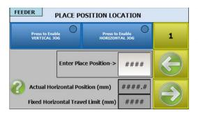
The Gantry transfers the board forward to the support table and stops at the Place Position Location.
