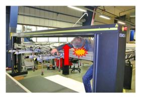
There is a risk of crushing/shearing between moving carriage beam and stack/gantry.
