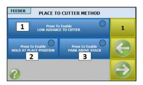
The feeder transfers the boards to the **Cutting Table** to a position where the leading edge of the board is approximately 150mm onto the cutter conveyor.
