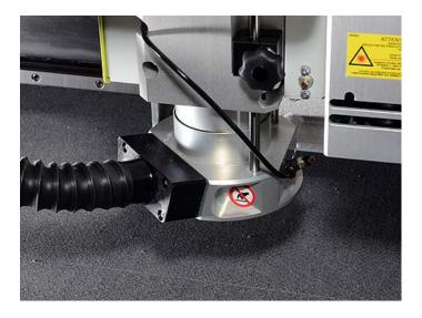
The **Vacuum Cleaner** can be used for automatic cleaning of the felt mat: Prepare program to make a file that covers the actual area. Set "bit size" to 65 mm (2.5 inch).
