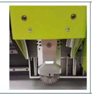
The **Dual HDU** HD Perf tool position is for 60 mm wheels, Perforation or **Crease**. The position is identified by the system as "HD Perf". It delivers the equivalent of 50 Kg [110 lbs.] downforce. The HD Perf position can handle cut depths up to 6 mm. This position was developed to deliver additional flexibility and to allow creasing and perforating heavy duty materials with the use of one tool unit.
