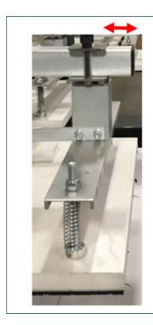
There has to be 35 mm/1.38 in. (arrow) from the plenum clamp to tip of pivot arm to maximize feed length.
