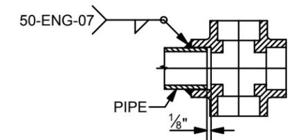
TYPICAL SOCKET WELD DETAIL
