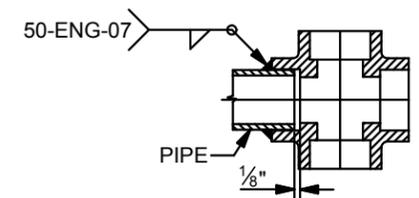
TYPICAL SOCKET WELD DETAIL
