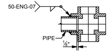
TYPICAL SOCKET WELD DETAIL
