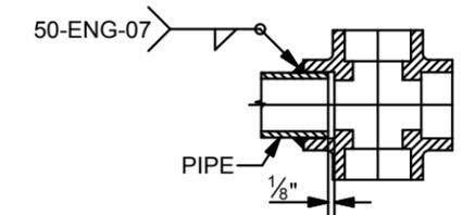
TYPICAL SOCKET WELD DETAIL
