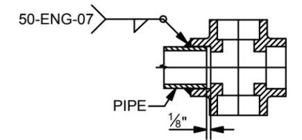
TYPICAL SOCKET WELD DETAIL
