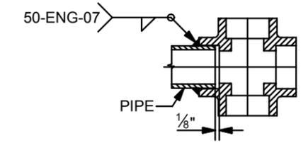
TYPICAL SOCKET WELD DETAIL
