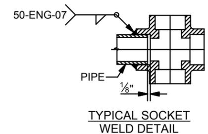
TYPICAL SOCKET WELD DETAIL
