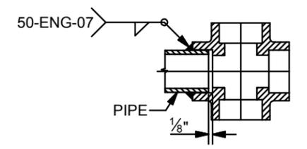
TYPICAL SOCKET WELD DETAIL
