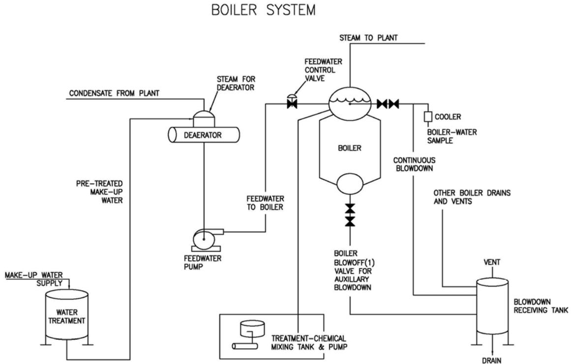
How much blowdown is required depends on allowable boiler water concentrations. It will be seen that:
