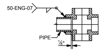
TYPICAL SOCKET WELD DETAIL
