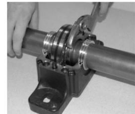
Figure 2) Tighten Until Snug
