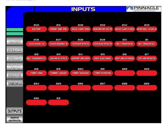
The Inputs screen shows indicators that depict the status of individual machine parts/functions.
