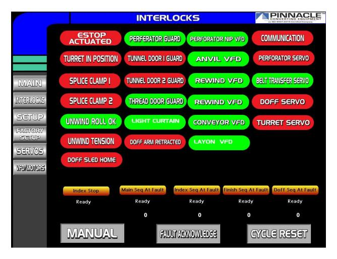
The GREEN/RED indicators display conditions of the machine that may prevent the machine from starting or cause the machine to stop. When any of these conditions occur, the condition must be cleared and the reset button on the machine must be pressed to start the machine again.
