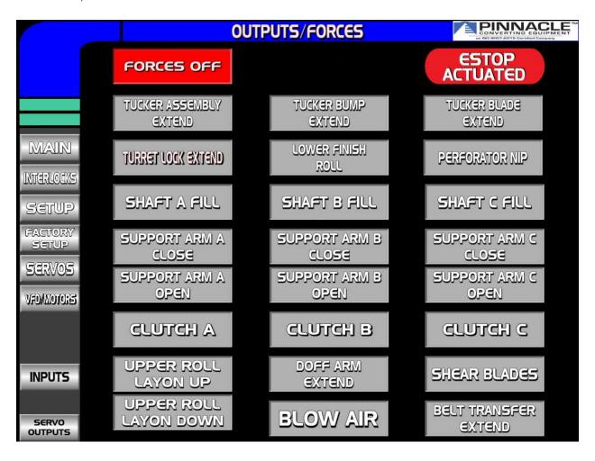
The Outputs screen allows the operator to manually actuate machine functions.
