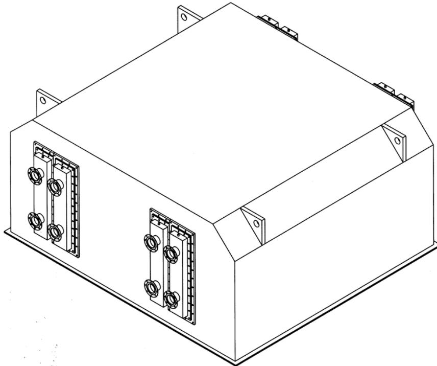
**Figure 2 - Shroud / Air Guide Cover**
