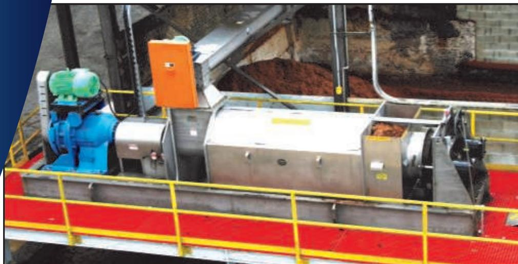
➔ **The VP-24 screw presses are used in dewatering tobacco stems and dust.**
