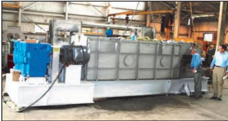
All of Vincent's screw presses can be made vapor tight and ATEX certified. This ← VP-24 is used in a pectin application.
