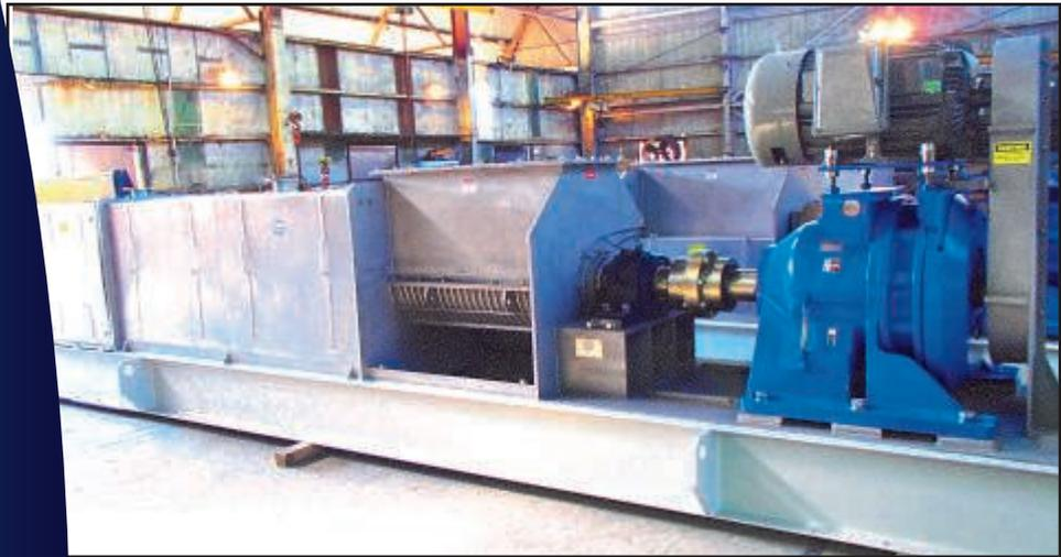
➔ **This VP-24 was built for Corn Wet Milling and is equipped with the optional inlet hopper screen.**
