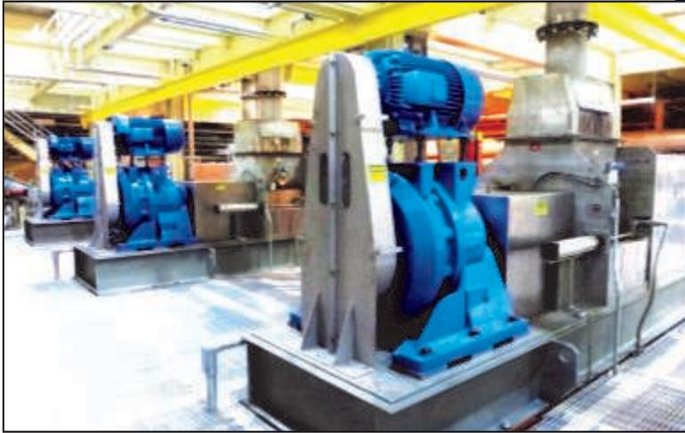
→ The VP screw press is used in both virgin and recycle mills to press waste streams and screen rejects.
