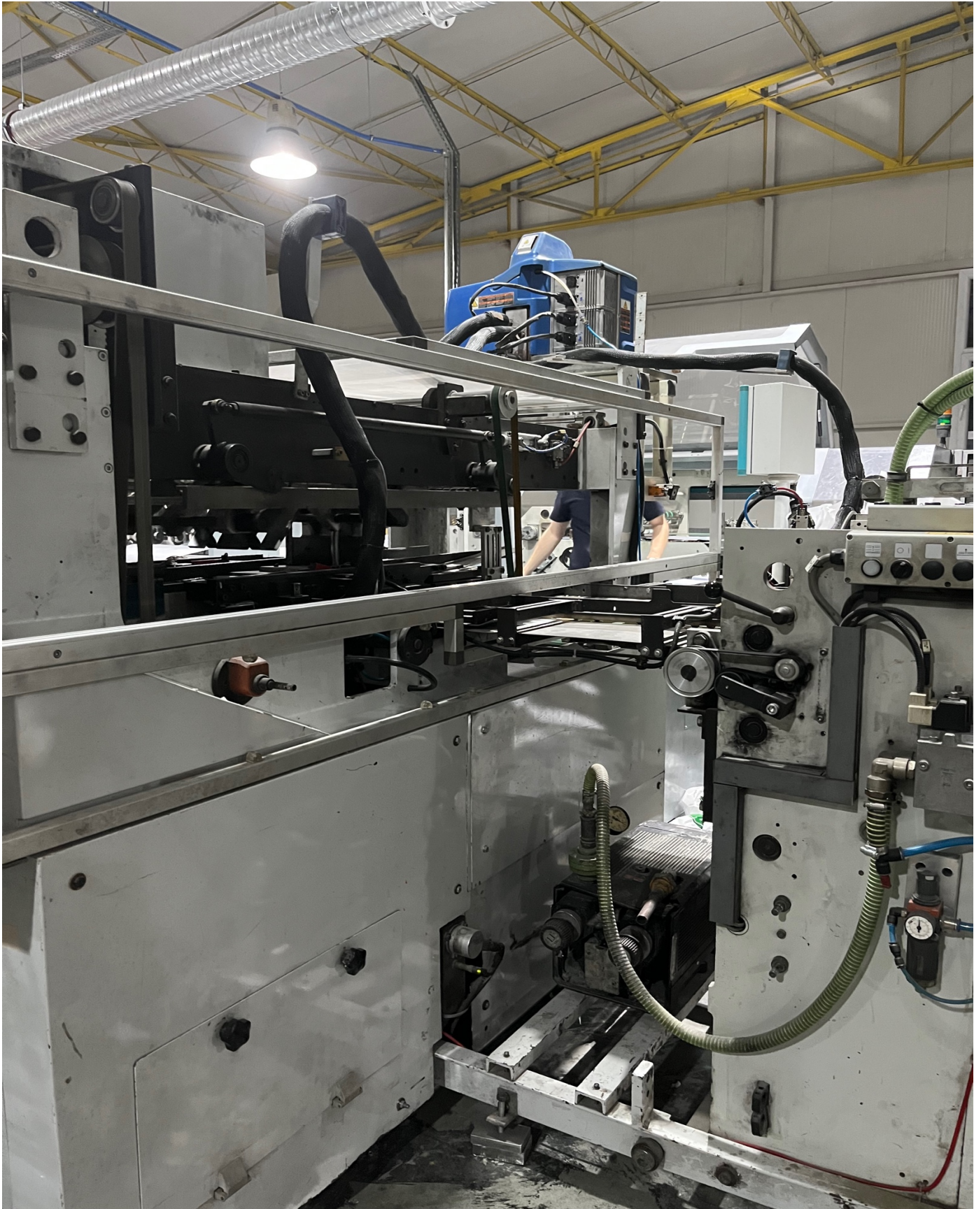
Wrapping machine is sheet-feed model with Heidelberg suction head
