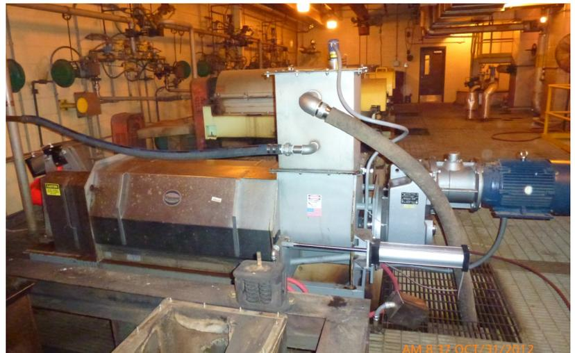
**KP-16 with Level Sensor for Speed Control**
