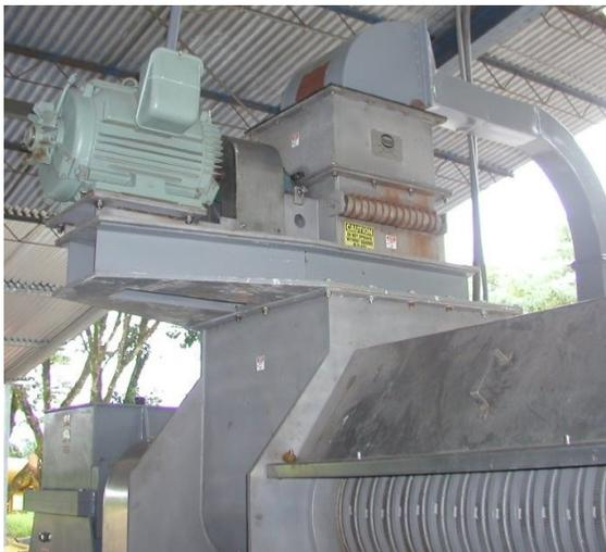
**Shredder at Press Inlet**
