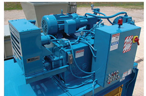
High-efficiency power unit and electrical disconnect.
