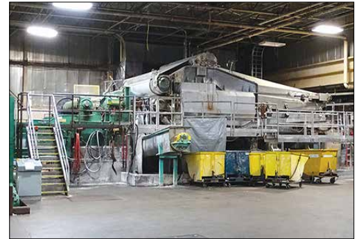
122" Metso Twin Wire Wetlap Machine 232 BDTPD
