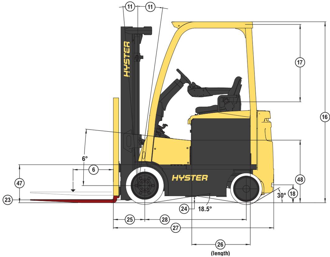
Circled dimensions correspond to the line numbers on the tabulated chart inside the technical guide. Dimensions are in inches (millimeters).
