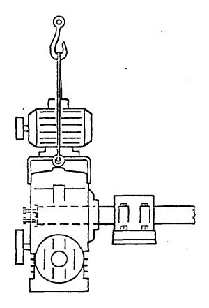
7. Remove cover, loosen the bolts for shrink disc and with a puller remove the gear box.
