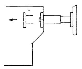
4. Loosen the flange and pull out the bearing and bearing housing.
