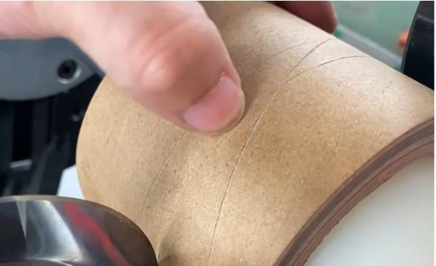
If the cutting line doesn't coincide, you can adjust the following screws to move the knife until they can cut in one line.
