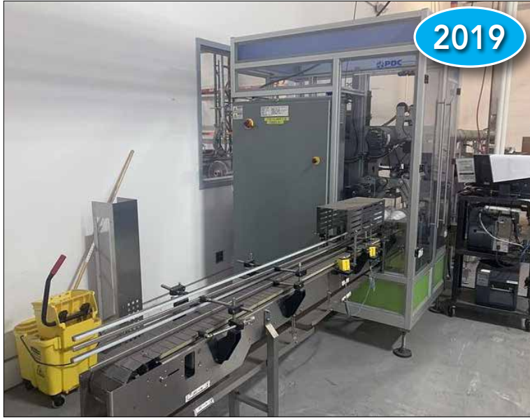
PDC Label Applicator and Steam Tunnel
