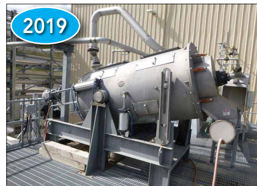
Vincent Model EF-30 Sludge Press S/S S/N 17590-8, Manufactured 2019
