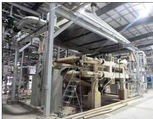
120" Rebuilt Press Technologies Heavy Duty 3.0m Twin Wire Wedge Thickener Model 120-WT
