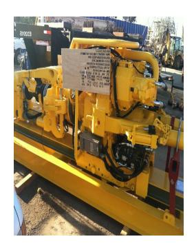
**TDH 250 BY NOV 3X HYD MOTORS** 750 H.P. 13.5 FT. LG. 13,200 LBS 18.71 TO 1 RATIO 230 RPM 25,000 FT LBS CONTINUOUS **40,000 FT LBS MAX TORQUE FOR DRILLING STATIC BRAKE 25,000 LBS** 2 ¾ INNER DIAMETER 5,000 PSI **50,000 LBS BREAK OUT** D.P. RANGE 2 7/8 TO 5 1/2 **IBOP RATING 10,000 LBS ROTATION UNLIMITED CRT READY- YES LIFT 250 TON**
