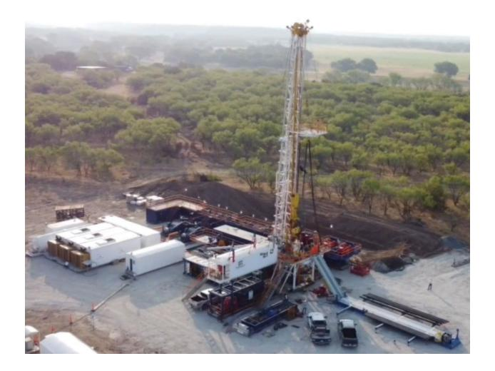
1000 HP Electric Drilling Rig
