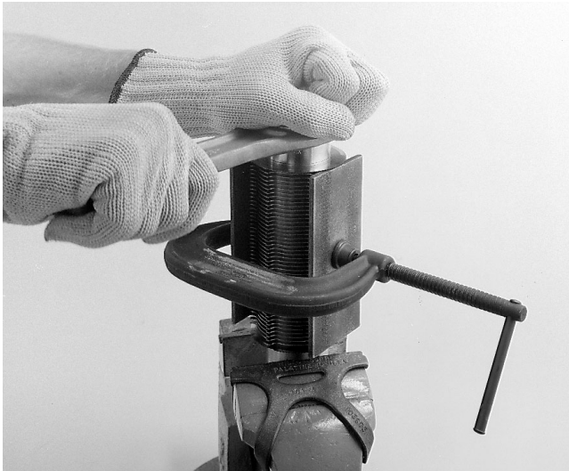
Figure 34 — Use spindle wrench to loosen and tighten the spindle nut. Shown above is a clamping method to align the feed discs while tightening the spindle nut.
