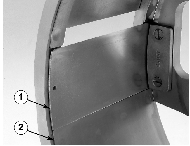
Figure 22 — Slicing knife properly seated. (1) Slicing Knife, (2) Inner Band of Slicing Case.
