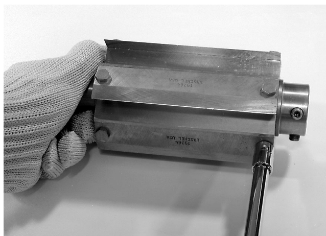
Figure 36 — Heavy duty crosscut knife spindle (stainless steel) disassembly
