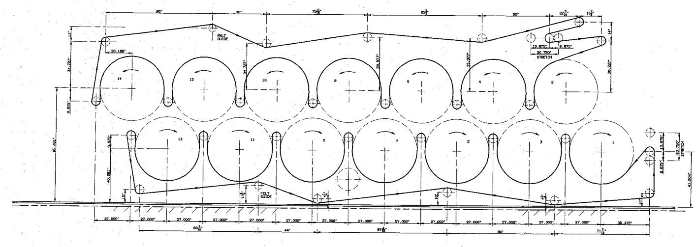
FIRST DRYER SECTION - PROPOSED FELT RUN
