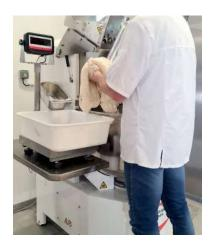
To further facilitate the operator's task, a mechanical device ensures that the arms always stop in the « opened » position whenever the equipment stops, thus giving better access for emptying or cleaning the tank.
