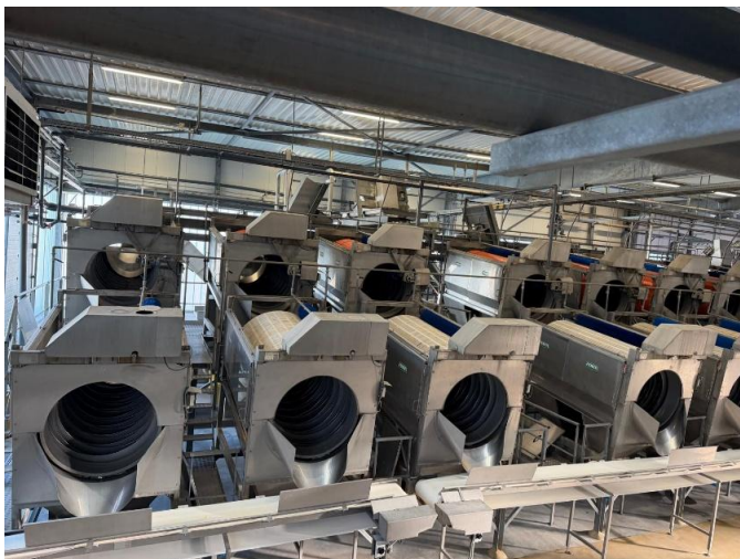
8x drums: cutting drums and spot cutters
