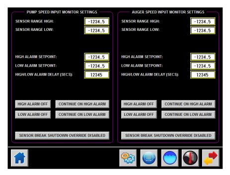
Each motor speed input has the following settings:
