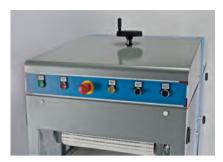
Independently variable speed for in- and outfeed belt, reverse button for last bread, height-adjustable upper infeed conveyer belt.
