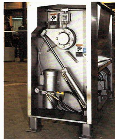
Tilt End - Oversized self-contained hydraulic system powers cylinders for smooth operation.
