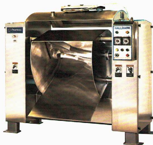
Tilt End - Oversized self-contained hydraulic system powers cylinders for smooth operation.
