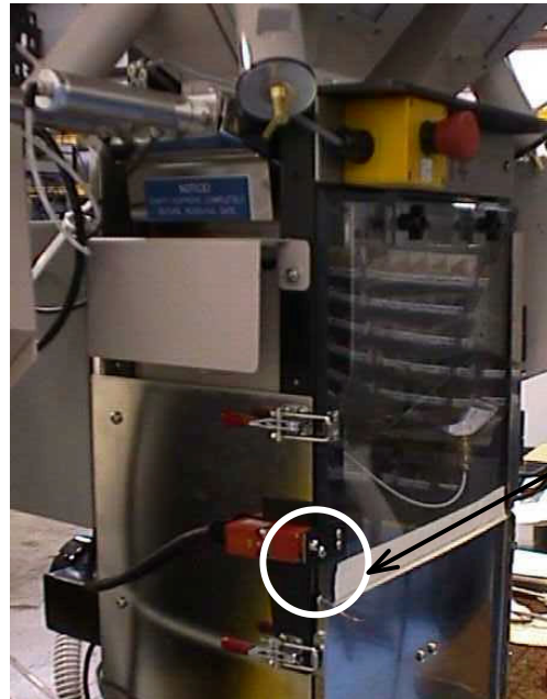
Electrical safety interlock switch (Located on mixer door)
