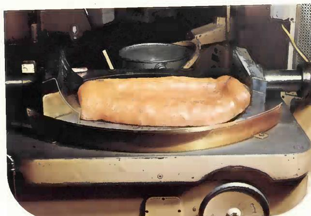
The working surface consists of a cooled rotating table, on which the sugar mass is kneaded by two opposed blades. These are also cooled. They fold and crush the sugar mass as the table makes regular 90° turns.
